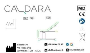
The electrical devices can be identified from the respective labels where the following data are reported:
